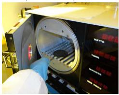
2. **Dehydrate** the wafer baking it in 150°C or 200 C hot plate for 5-10 mins
