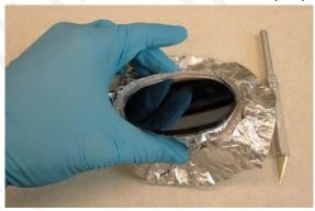
10. Finally, peel the PDMS mold from the master
