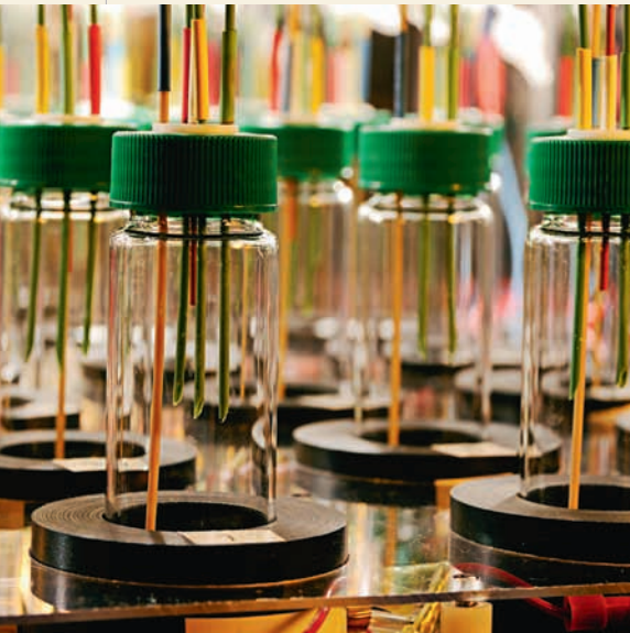
A custom fluidic system maintains bacteria being challenged by drug treatments.
