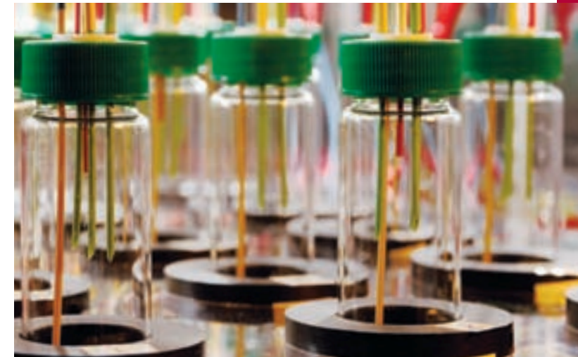
A custom fluidic system maintains bacteria being challenged by drug treatments.
